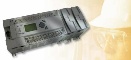
MicroLogix 1400 from Rockwell Automation complements the existing MicroLogix family of small programmable logic controllers, by combining the features you demand from MicroLogix 1100, such as Ethernet/IP, online editing, and a built-in LCD, plus enhanced features, such as increased I/O, faster High Speed Counter/PTO and communication capabilities.
